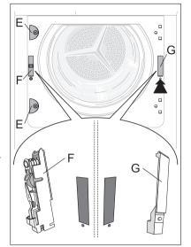
**Note regarding contact protection:** The machine is only secure for operations again once all plastic parts have been inserted.
